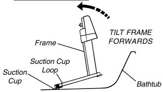
FIGURE 2 - REMOVING THE FRAME FROM THE BATHTUB
